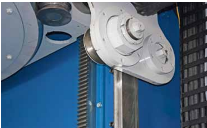
The toptable, rollerhead drive, and bellbacker are roller-guided and cantilevered from the ePak's rigid uniframe with zero gap component movement, eliminating vibration for fast and smooth operation
