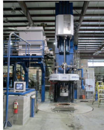
Figure 7: The uniframe ePak main tower eliminates the support legs found on most packerhead pipe production systems, allowing the use of a smaller turntable and free access to molds and other system components. At left, the ePak control PC is Windows based for intuitive operation of the entire pipe production cycle.
