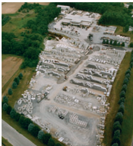
Figure 1: The 20-acre Coastal Pipeline Products facility features a 30,000 square foot main building housing all dry cast production as well as a portion of the wet cast operation. The majority of wet cast products are produced outside, except during inclement weather.
