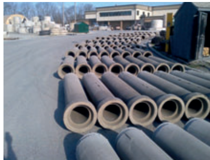
Figure 2: Coastal Pipeline Products produces pipe from 12 to 72 inch inside diameter. Here, recently "tipped out" 15-inch pipe is laid out in preparation for yarding.
