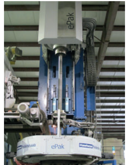
Figure 5: The eDrive system found in the ePak packerhead pipe production system from HawkeyePedershaab features two gearless permanent-magnet electric motors (top section in photo above) that provide direct control of the packerhead torque and speed and help reduce maintenance and energy use. Dry mix concrete is fed into the pipe form by a troughed conveyor through the Top Table Assembly (at bottom of photo).
