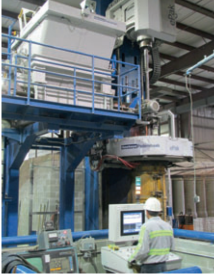
Figure 4: The HawkeyePedershaab ePak RCP production system at Coastal Pipeline Products features PC- and PLC-based controls that continuously monitor and adjust all pipe production variables, including concrete feed rate, crosshead lift with variable speed, packerhead shaft torque, bell packer lift speed, top table control, turntable control and concrete feeder water spray. The automatic control system stores all mix recipes, machine settings for each pipe size, and production history record for every pipe produced. In this photo, the elevated bin on the platform directly in front of the operator is a 3-yard Concrete Feeder that holds the dry mix concrete coming from the mixer and feeds it at a precise rate as needed by the ePak packerhead system, seen just to the right of the Feeder.
